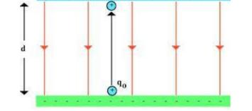
Let us consider a positive charge +q is placed in an electric field at point B. If the charge is allowed to move freely, it will acquire kinetic energy and will move from B to A. Conversely, we can say that an external force is required to keep the charge at rest or to move with uniform velocity from A to B. (1)
