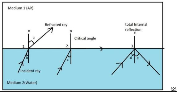
Total internal reflection occurs when light traveling from a region of a higher index of refraction to a region of a lower index of refraction strikes the boundary at an angle greater than the critical angle such that all light reflects back into the region of the higher index of refraction. (1)
